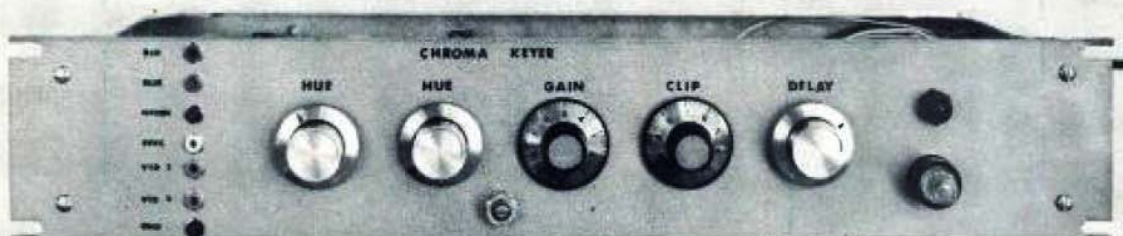
Fig. 2 Coarse hue control is at left, fine hue is second control from left. Balance adjust is between fine hue and gain controls.
